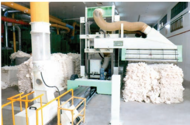
A view of newly installed “LMW Swift Floc LA21” Bale Plucker machine in our OE Hall at Rajapalaiyam.
