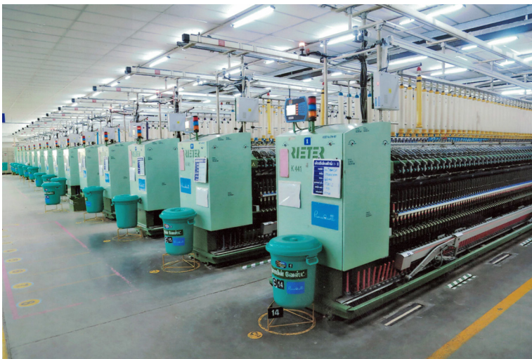
A view of the “Rieter K441 Compact Spinning Ring Frames” in our Mill at Rajapalaiyam.
